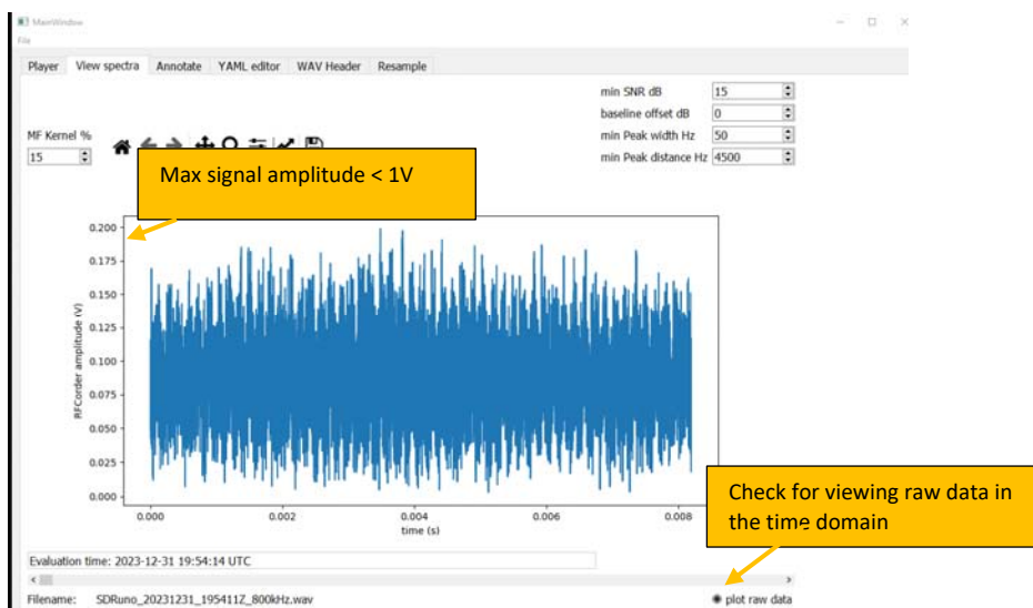
Fig. 1-27: Checking for correct signal amplitude e.g. when setting the gain before resampling. The signal values need always to remain below 1V to prevent clipping. It is recommendable to leave some margin for reducing intermodulation artifacts.
