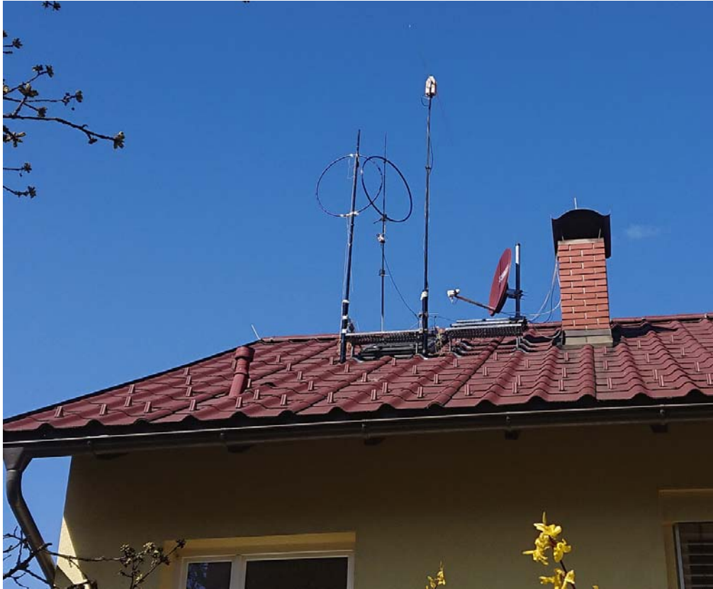
Fig. 3-20: Active dipole and two loops mounted on spiderbeam telescope masts on the roof.
