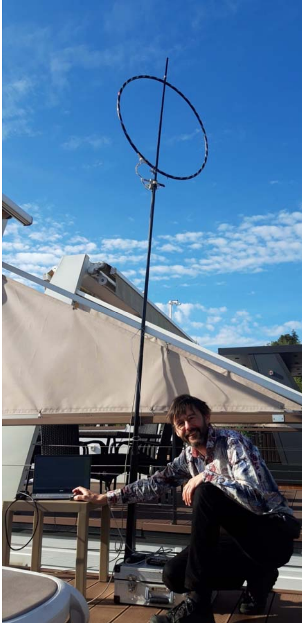
Fig. 3-19: Deployment Wellbrook 1530Flex with homemade loop on a houseboat in Portoroz (Slovenia) 2023. The amplifier part is the small box just below the loop, the bias tee and power supply are on the case on the bottom.
