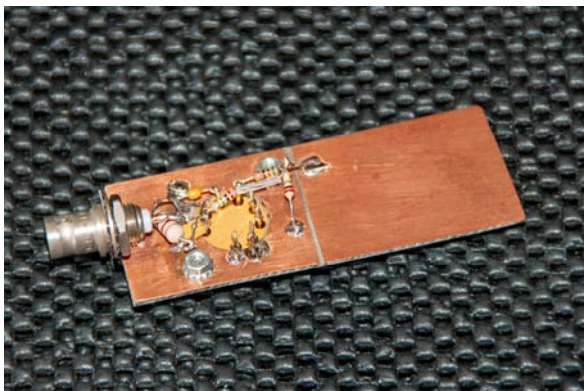
Fig. 3-14: Board of the whip antenna nr. 2 by S. Roberts
