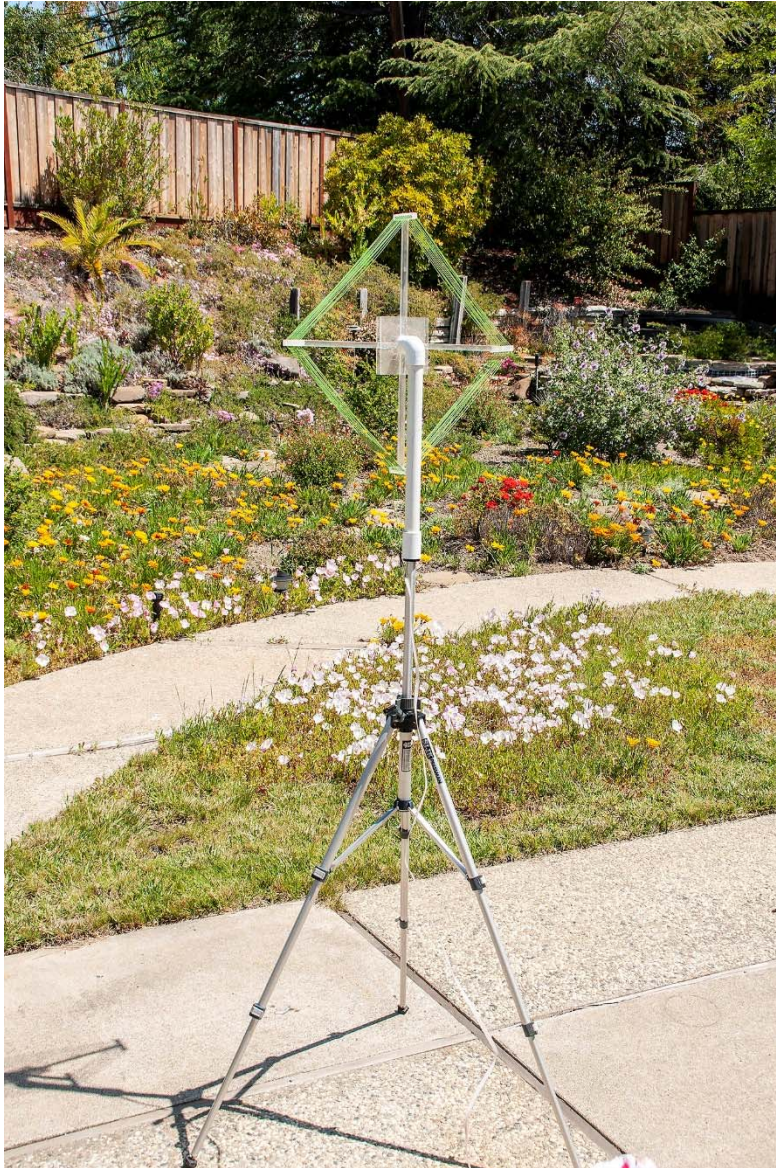
Fig. 3-16: Loop antenna used by S. Roberts
